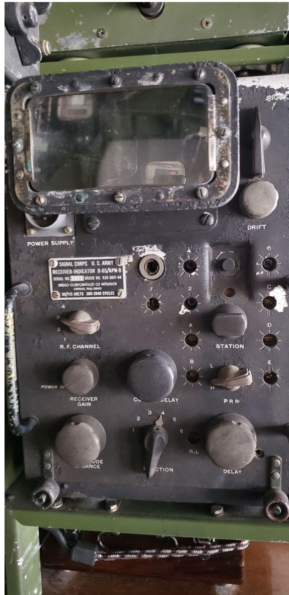
The R65 APN-9 in a Boeing B-17G
